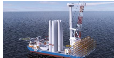
WTIV (Wind Turbine Installation Vessel)
